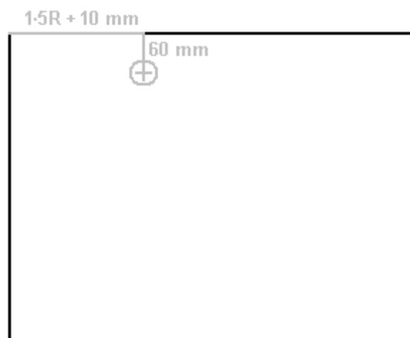
Mark a bearing circle, cut it out and insert the second bearing into that hole. Place a piece of axle material (or a length of dowel of exactly the same diameter) in the bearing and position the first side so that the axle material passes through both bearings, aligning them exactly. Mark around the edges of the first side, being very careful when marking the edge which will become the base of the second side:
