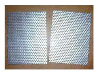
Your local steel supplier probably has some types on hand and can let you see how flexible a particular variety is. The shape shown above is for a "three plate per cell" design where there are two active plate faces. Ideally, you want two to four square inches of plate area per amp of current flowing through the cell, because that gives very long electrode life and minimum heating due to the plates.
