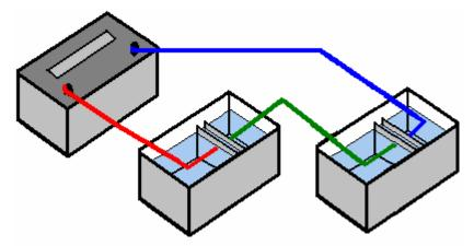
This arrangement uses our 1.24 volts twice while the twelve volts stays unchanged and so the electrical efficiency goes up to 20% and the heat loss drops to 80%. That is quite an improvement but even more important is the fact that twice as much HHO gas is now produced, so we have doubled the electrical efficiency **and** doubled the gas output, giving a result which is four times better than before.
