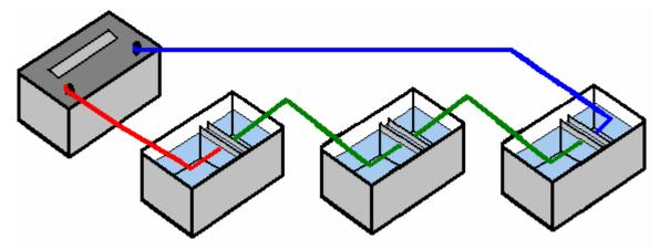
This time we are using three of our 1.24 volt sections and this gives us an electrical efficiency of 30% and three times the amount of gas, making the system nine times more effective.
