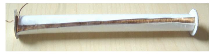
That process is repeated until all of the desired layers have been wound. Finally, the wire is cut with a few inches left for connecting the coil in the circuit, and the wire is passed through a second hole in one of the flanges:
