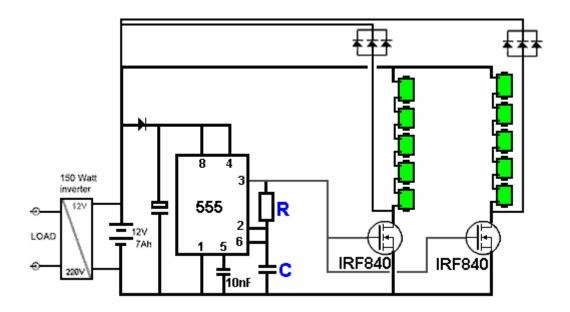
The resistor "R" and the capacitor "C" control the frequency of the pulsing and the result is very good. However, as the developer has powered both coil chains of his rotor circuit from a single transistor (although they generate at least 600V feedback pulses), he used just one transistor for his tests. He also likes to use his circuit which swaps over two drive batteries, one to provide current while the other one is recharging, but that is a minor matter.
