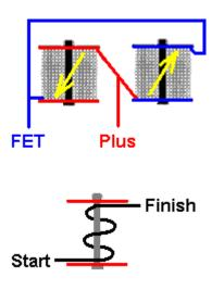
The two sets of five coils in series are connected in opposite directions as shown above. The Start of the set of coils shown in blue and the Finish of the set of coils shown in red are connected to the Plus of the battery. This causes current to flow in opposite directions in each set of five coils and if one set has a North pole facing the rotor, then the other set will have a South pole facing the rotor. The coils are alternated around the rotor like this:
