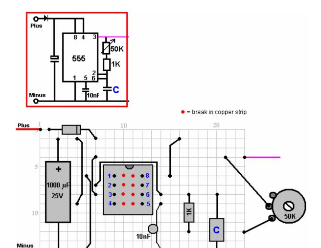
The capacitor "C" will be about 10 nF and the variable resistor can be 47K or 50K linear or a higher value could be used.
