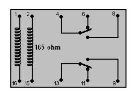
This is the electronic version of a mechanical two-pole switch. A brief pulse of current between pins 1 and 16 locks the switch in one position and later, a pulse of current between pins 2 and 15 locks it in the other position. The current drain on the circuit would be almost zero.
