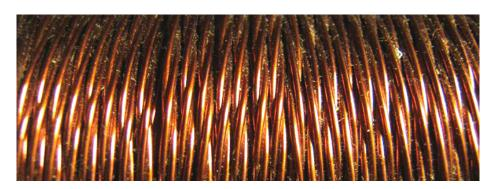
This completed coil now contains three separate coils in very close proximity to each other and that arrangement is excellent when one coil is powered up, for inducing energy in the other two coils. This winding now contains coils 1,2 and 3 of the circuit diagram. There is no need to concern yourself with marking the ends of each strand of wire as a simple ohmmeter will tell you which two ends have a winding between them.
