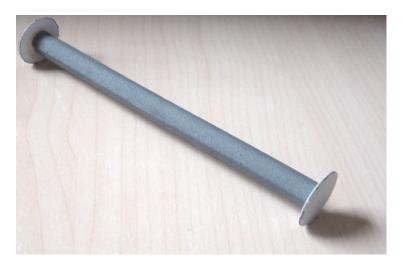
Cut a 140 mm wide piece of paper 32 mm long. This width matches the gap between the spool flanges. Attach a strip of Selotape to the paper so that it overlaps by half its width all along the paper strip and set it aside until the first layer of wire has been wound.
