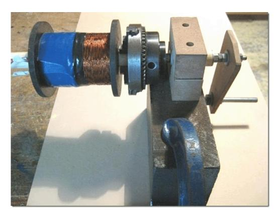
The three strands of wire which form coils "1", "2" and "3" are 0.7 mm diameter wire and they are twisted together to become a "Litz" wire before being wound into the coil "B". This produces a much thicker composite wire strand which is easy to wind accurately on to the spool. The winder shown above uses a chuck to grip the coil core for winding, but any simple winder will work well.
