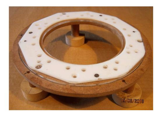
The small coils are held in place with cable ties and are easy to remove. Each coil has a resistance of 0.8 ohms and the cores are standard 6 mm diameter galvanised iron bolts which do not retain magnetism, that is, they do not become permanent magnets no matter how often they are stroked repeatedly with a strong permanent magnet. The set of ten coils mounted around the rotor look like this:
