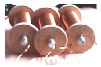
Three of these coils can be wound from a single 500 gram reel of 0.71 mm wire and the iron cores can certainly operate at more than 6000 Hz. Each of these coils has about 315 turns and a DC resistance of 1.6 ohms. However, ferrite is generally considered to be a better core for high frequency operation
