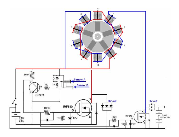
As it stands, this circuit can charge 12V or 24V batteries or power a 12V inverter connected across a 12V battery, or 24V inverter connected across a 24V battery. A version of this circuit with fewer components which works very well indeed is this:
