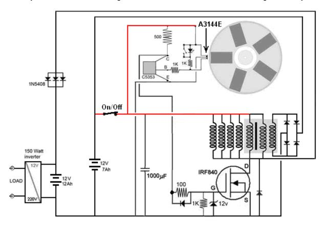
Here, the battery which powers the inverter which supplies the load is increased in capacity and while the developer used two of his 7 Amp-Hour batteries, you can use a standard 12-volt 12 Amp-Hour
