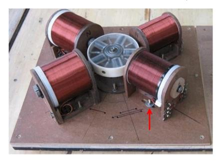
Notice the way that the coil mounts allow the distance between the coils and the rotor to be changed. The working gap between the rotor and the coils can be adjusted so that the performance can be maximised by finding the most effective gap.
