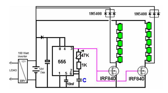
This arrangement allows for considerable alteration of the operating frequency by merely turning a knob. Experienced constructors will have their own preferred methods of construction, but we might choose to use a layout on an open board in order to make it easy to see what is happening and to give good cooling during the development stage.
