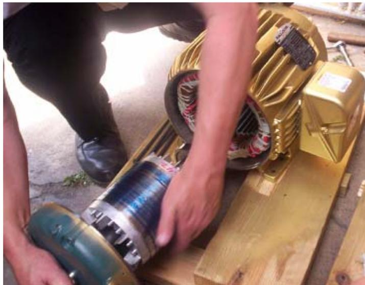
The second end-plate is then removed and placed on the opposite end of the stator housing:
